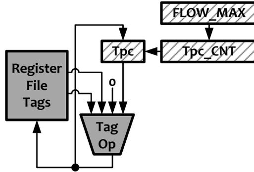
Figure 6.13: The additional components (in stripes) for the tunable propagation of the baseline DIFT system.
