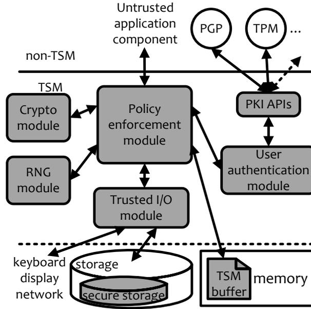
Figure 4.4: TSM architecture. The trusted (gray) parts of the system are the TSM and the SP-protected secure memory and secure storage.
