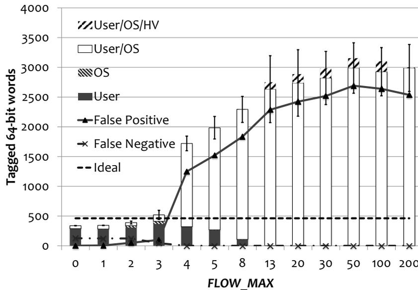
Figure 6.14: False positives and false negatives analysis after running the  $\pi$ -calculation program. The contributions from the hypervisor (HV), User/HV and OS/HV are all zeroes and not plotted on the graph. The x-axis denotes different settings of the  $FLOW\_MAX$  values and the y-axis shows the number of tagged 64-bit words in the system. Note that the  $x$ -axis is not in linear scale.
