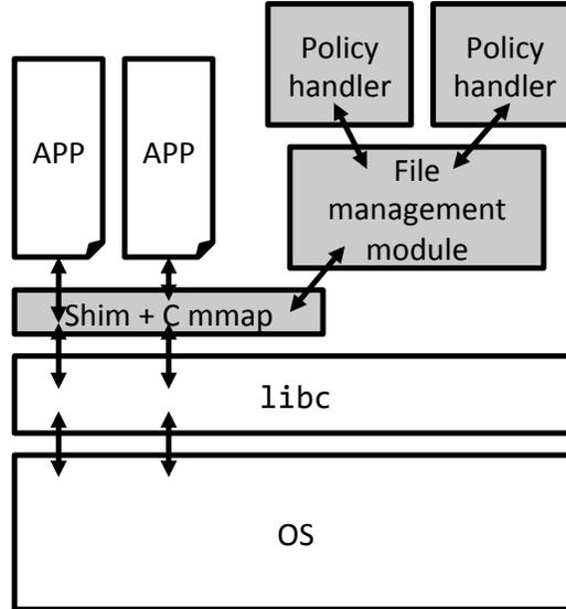
Figure 5.8: The C shim implementation for the DataSafe file access redirection.
