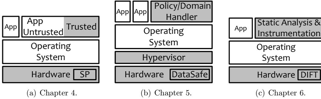
Figure 3.1: The differences between the Trusted Computing Base (TCB) of Chapters 4, 5 and 6. Gray components constitute the TCB, whereas white components are untrusted and can be exploited by attackers. The hardware blocks SP, DataSafe and DIFT are explained in detail in Chapters 4, 5 and 6, respectively.
