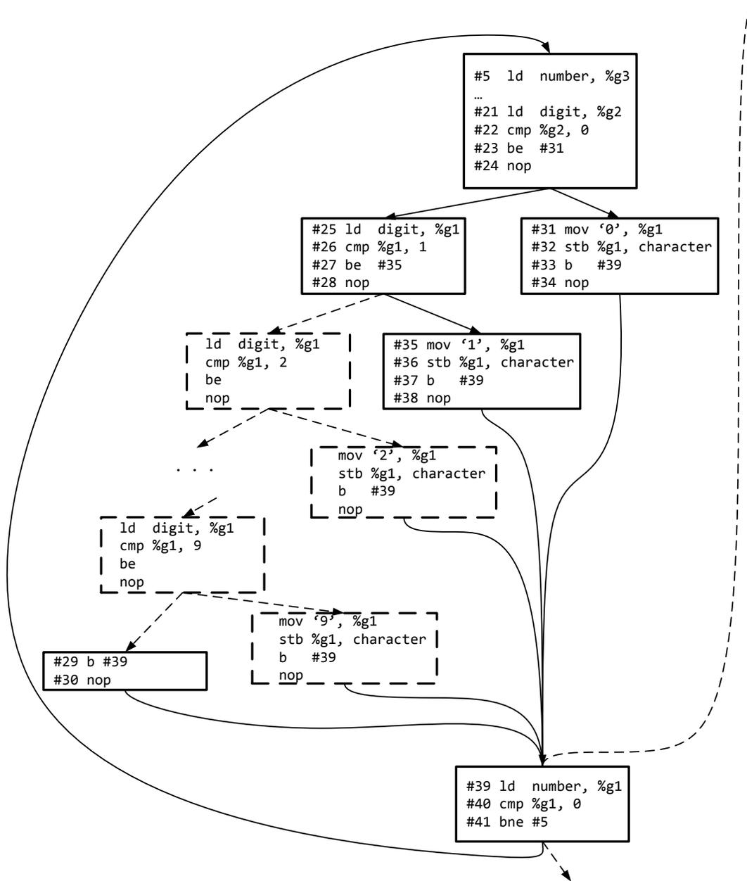
Figure 6.12: The control flow graph of the core function of `sprintf()`. Each block has its corresponding line numbers from Figure 6.11. Note that in this particular example, an ideal `FLOW_MAX` value would be 3, to cover the sequence of `nop`, `move` and `stb` instructions after the tagged branches (`be`) in line 23 and 27.
