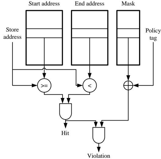
Figure 5.10: The DataSafe output control hardware component.
