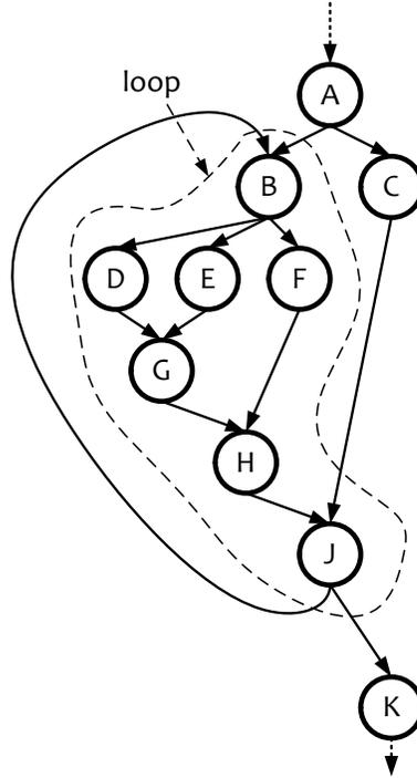
Figure 6.5: An example control flow graph to illustrate the loop peeling of Algorithm 3.
