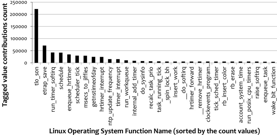
Figure 6.15: The Linux operating system functions that contribute to the tagged values in the system. Each write of a tagged 64-bit word to the memory by the operating system is counted as one contribution. The list is sorted by the amount of contribution from the various operating system functions.
