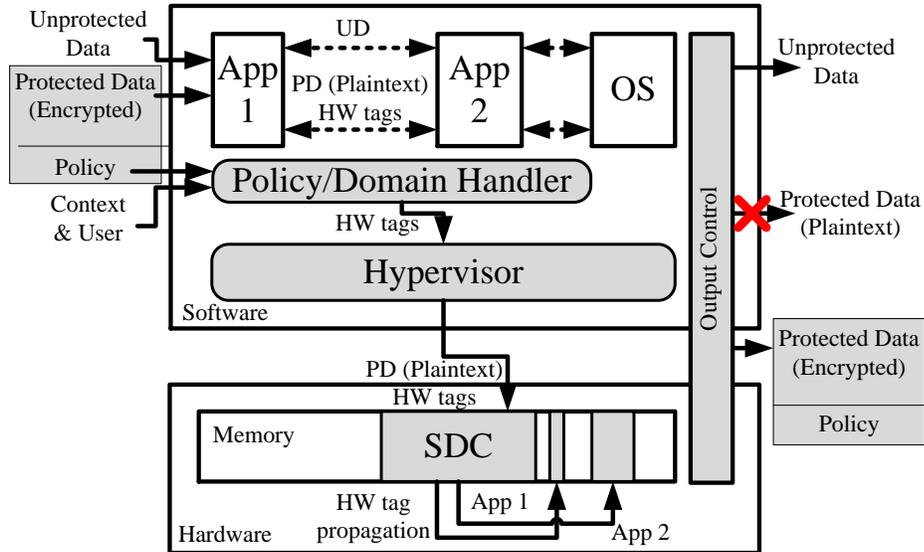
Figure 5.2: Software-hardware monitoring of Protected Data (PD) in DataSafe architecture. Unprotected Data (UD) is unchanged. Since the hardware tags of the Protected Data are tracked and propagated at the physical memory level by the hardware, this allows seamless tracking across applications (and across application-OS boundaries), as illustrated by the top row of boxes. (Gray indicates DataSafe additions).
