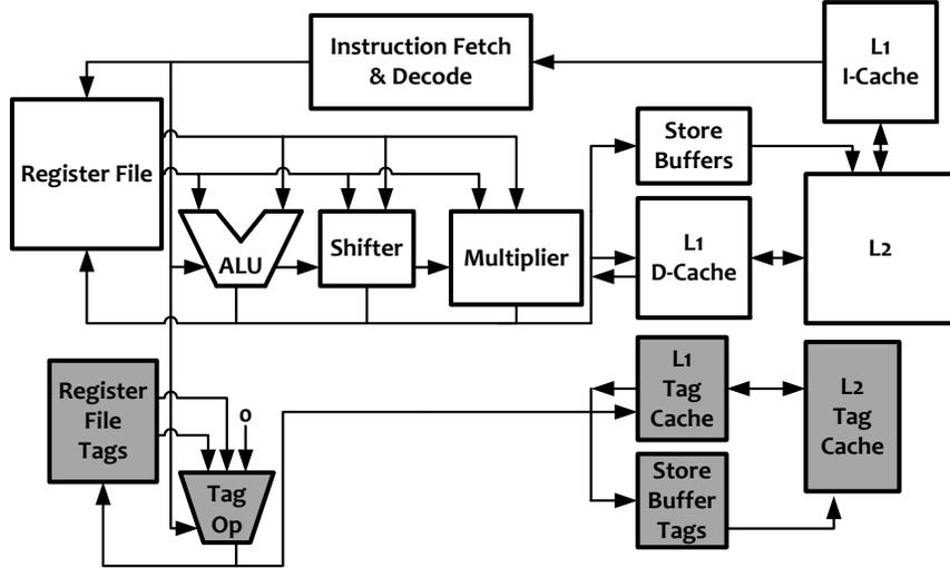
Figure 6.3: The baseline hardware DIFT architecture. The white blocks are basic processor components whereas the gray blocks are DIFT components.
