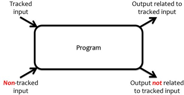
Figure 6.1: A high-level view of tracking information flow in computer programs. The goal is to be able to distinguish whether or not the program’s output is related to the input that we wish to track.
