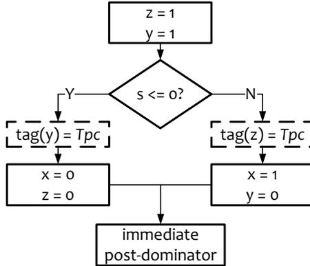
Figure 6.7: The instrumented control flow graph of the conditional execution example after the compensation for tag assignments to account for the untaken path in the dashed boxes.
