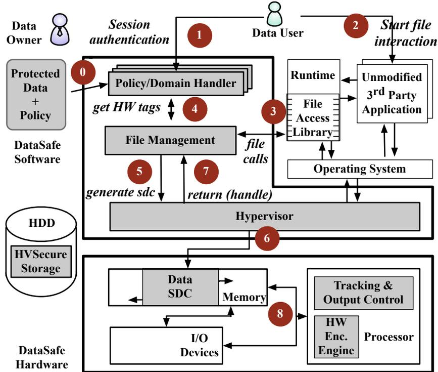
Figure 5.3: The software and hardware components of DataSafe. The gray parts are new and trusted DataSafe components, while the striped file access library is modified but untrusted. All other software entities including the unmodified third-party applications and the operating system are assumed to be untrusted.
