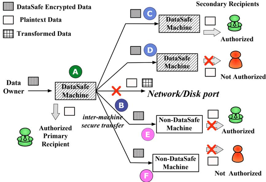
Figure 5.1: DataSafe architecture protects data confidentiality across machines (new and legacy) and users (authorized and not authorized).
