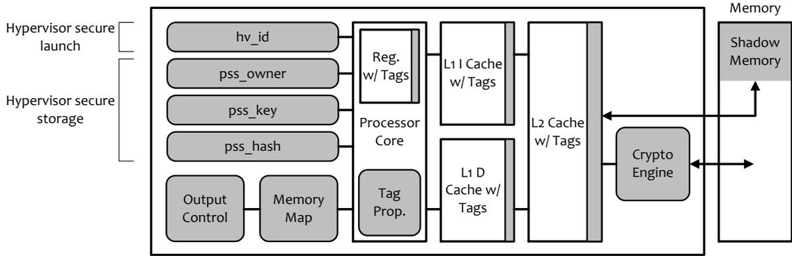
Figure 5.5: The DataSafe hardware components (gray).
