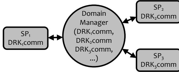
Figure 4.5: The pair-wise communication between the domain manager and the individual TSMs on different SP devices. Each SP device has its own unique  $DRK_i$  and  $DRK_i,comm$  denotes the symmetric communication key derived from the DRK to encrypt the communication data.
