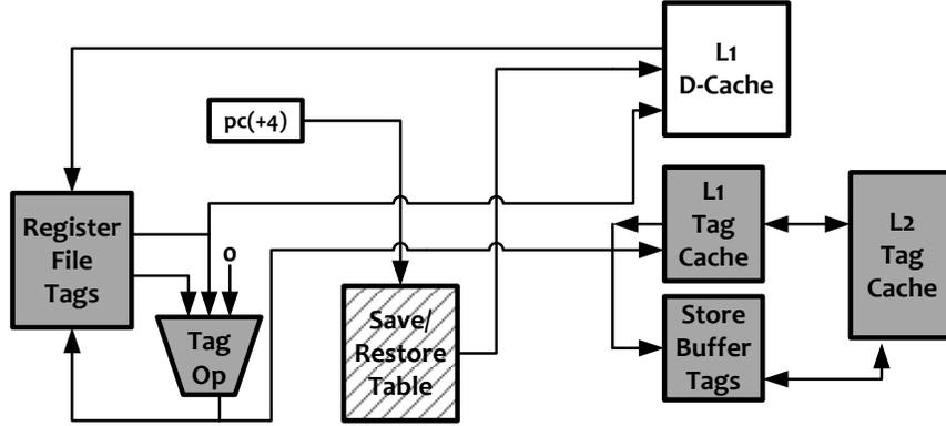
Figure 6.16: Additional DIFT components for register file tags save/restore (in stripes) to address tag pollution in the OS space.
