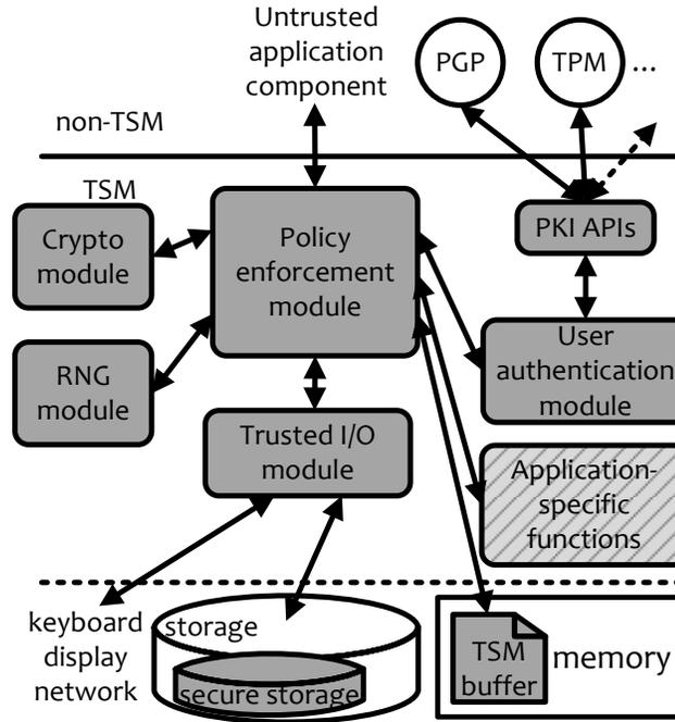
Figure 4.9: The TSM architecture including application-specific functionalities (shown in lighter gray with stripes).
