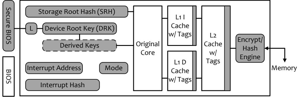
Figure 4.2: The internal components of a SP processor [37]. The derived keys block is enclosed in dashed line since it is not a real hardware component, but to show that the original core does not directly access the value of the DRK.
