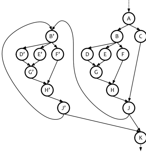
Figure 6.6: The modified control flow graph after loop peeling of Algorithm 3.
