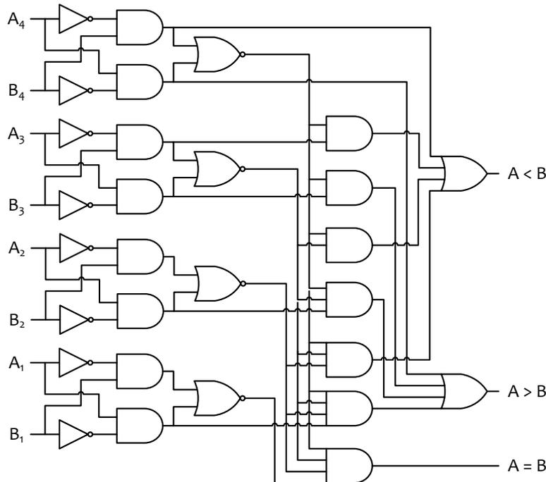
Figure 5.11: A typical logic design for a 4-bit magnitude comparator (from [82]).
