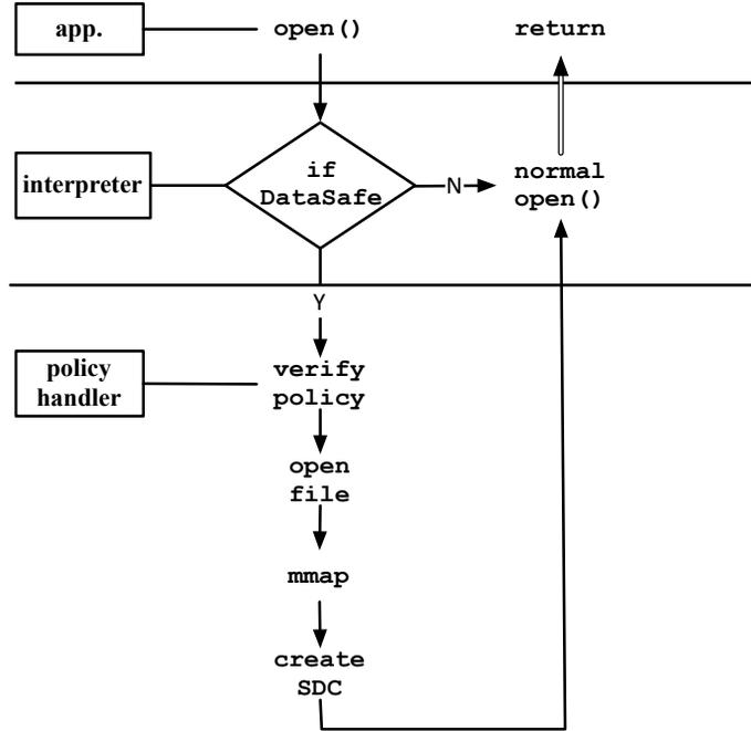
Figure 5.7: The file access redirection performed by DataSafe’s file management module in the Ruby language.
