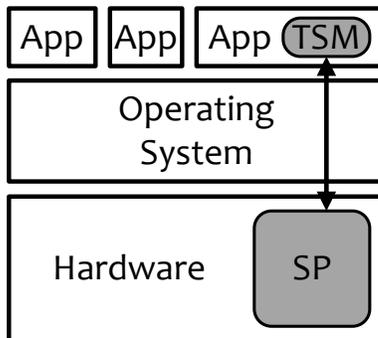
Figure 4.1: High-level view of our proposed solution. The white parts are the commodity computer system (untrusted) and the gray parts are the trusted part of an application (TSM) and the SP hardware components.
