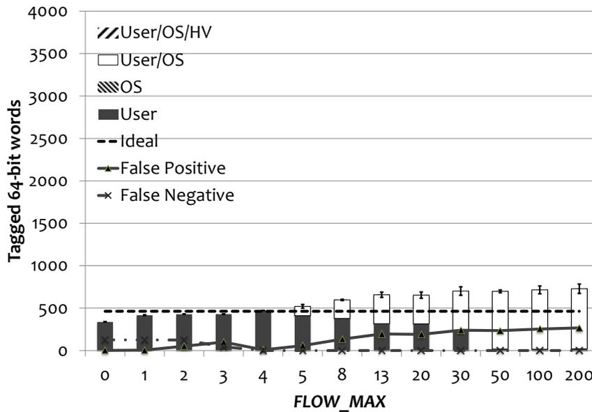
Figure 6.17: False positives and false negatives analysis after running the  $\pi$ -calculation program, with the register file tags save/restore mechanism. Note again that the  $x$ -axis is not in linear scale.
