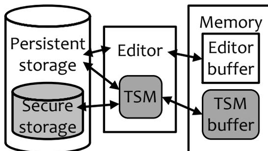
Figure 4.7: Partitioning an editor application into untrusted (white) and trusted (gray) parts. The TSM gets its own buffer to work with temporary decrypted data, and it can access both the secure storage where the policies are stored and normal storage where the protected (encrypted) content is stored.
