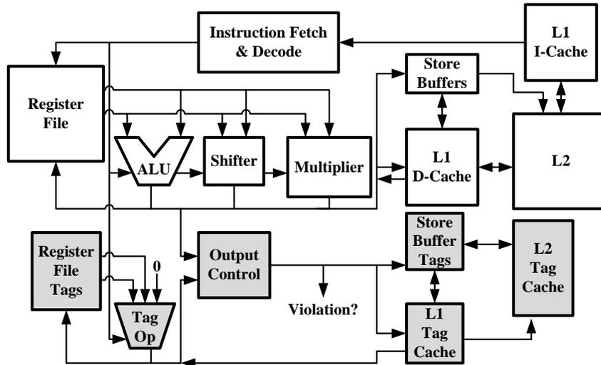
Figure 5.9: One possible implementation of the DataSafe information flow tracking processor architecture. White boxes are existing components while grey boxes are new.
