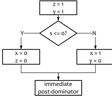
Figure 6.4: The control flow graph (CFG) of the conditional execution example. A node  $p$  post-dominates a node  $a$  if all paths to the exit node of the graph starting at  $a$  must go through  $p$ .
