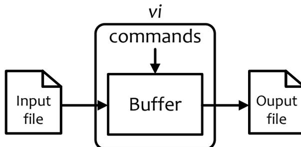
Figure 4.6: A simplified view of the *vi* program. *vi* reads in the input file and puts the content in the temporary buffer to manipulate it according to the commands from the user. *vi* commits to the output file from the buffer.
