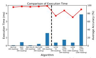
Figure 3: Execution time and accuracy of detection algorithms. The red line stands for the average accuracy. The maximum execution time for inferencing, using any of the ML/DL models shown, is 4 ms, much smaller than the 20 ms interval between new sensor measurements.
