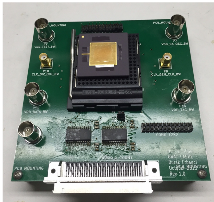
Figure 78 PCB used for testing of Newcache testchip.
